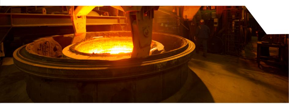
Our rapid pump-down allows for smaller temperature losses and an overall longer low vacuum phase, thus lowering the cost for overheating the melt in the LF and increasing the quality by longer fine vacuum treatment times.
