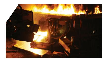
MTAG Switzerland's Robotemp is mounted on the floor next to the EAF so that both measurements and samples can be taken through the furnace door without changes to the EAF and so cartridges can be exchanged in the safe parking positions.
